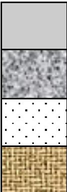
**Void** - simulation of regions starved of adhesive, circles machined through-the-thickness of the adhesive layer
