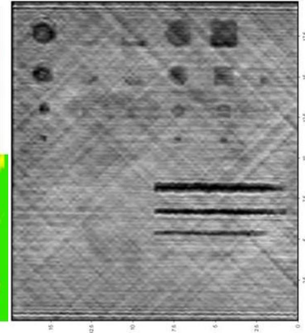
**Microwave of thick bond-line containing artificial defects (24 GHz)**
