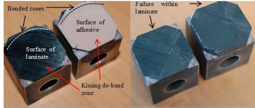
Note: Non-defective material failed in one of the parent laminate at 42 MPa, indicating that the adhesive bond strength was superior to the interlaminar (through-thickness) tensile strength of the laminate
