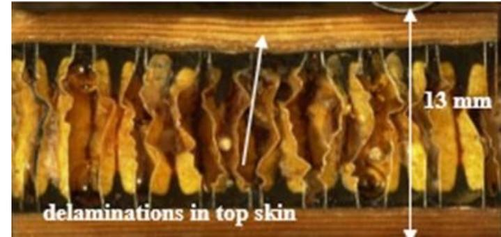
**Skin-to-core de-bond in GFRP/PU foam sandwich construction**
