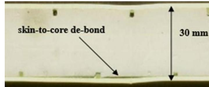
**Core crushing of CFRP/Nomex construction**
