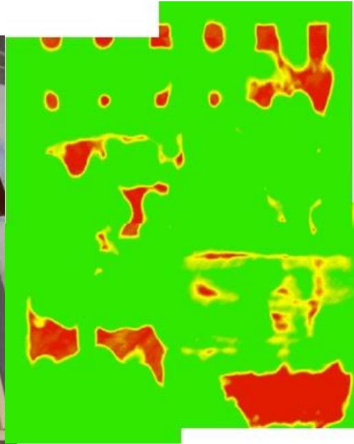
**1MHz thru-transmission ultrasonic c-scan**
